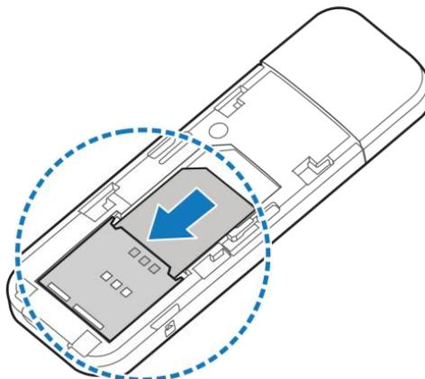
**IMPORTANT:** Your device supports a Standard (2FF) SIM card only. Do not use a Micro SIM with an adaptor as this may damage your device.
